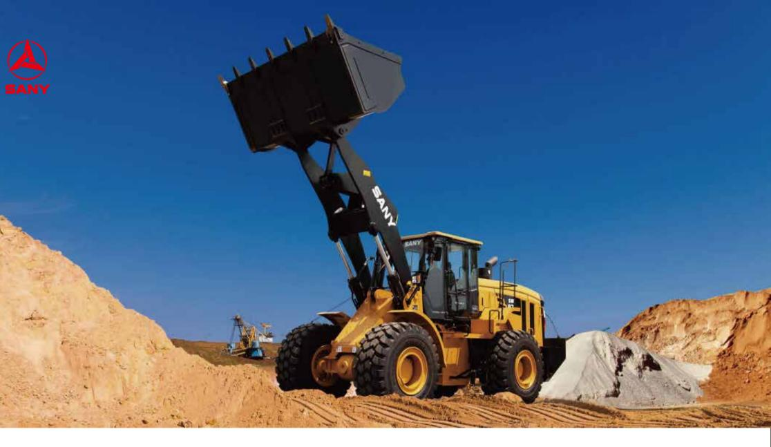
**Reliable, High-productivity & Smart** Rated power: 210 kW @2200 rpm | Operating weight: 24,300 kg | Rated payload: 7,000 kg Bucket capacity: 5.0 m<sup>3</sup>
